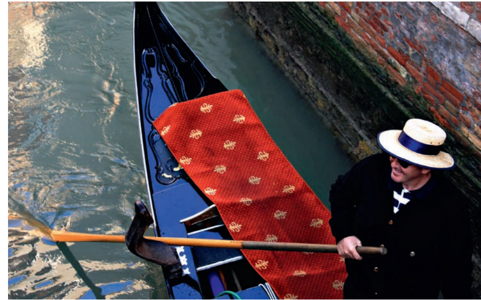
The asymmetry of the gondola means you can row it from only one side. FOTO: ZACH CROCKER
